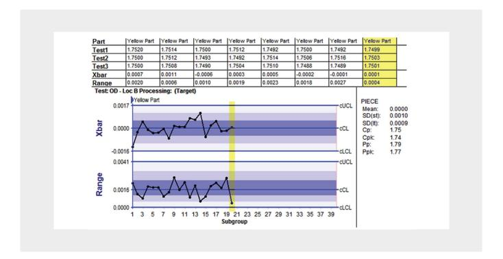
If we start making the blue part on the same machine, we can simply add the blue part data to our Target Xbar-R chart as shown below. ProFicient's "on the fly" processing option allows the user to easily combine data on the same chart and apply the deviation from target option at any time. The user can switch between Traditional and Target processing with the same set of data.
