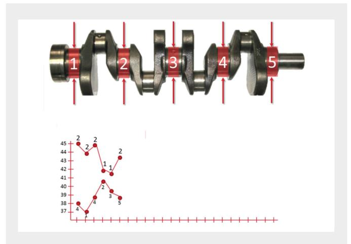
Note: The group chart is intentionally missing control limits because sometimes group charts are used for plotting dependent data streams.
