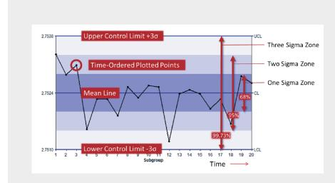
Note: Control limits are based on observed process data, not on specification limits. Lines on a chart representing 75% of the specification limit are not statistical control limits. Control limits may not always be centered on target or within the specification limits.
