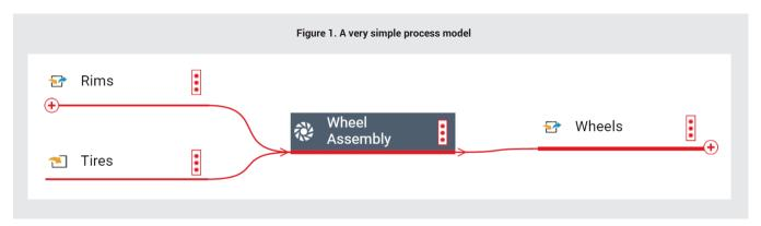
The process model simplifies root cause analysis in the manufacturing process. An inspection performed at the end of the production line allows the operator to perform checks or measurements and attribute the results to the appropriate process without requiring individual selection of components or processes. As a result, operators can spend more time doing other work, without sacrificing process or product quality.
