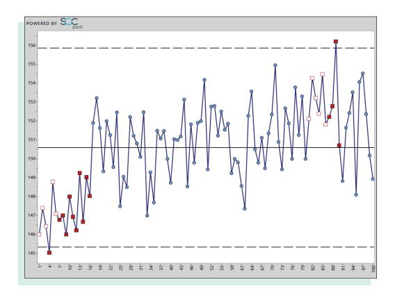
Without this determination of stability, any reliance on Cpk values is premature. The first issue to be addressed is getting to a stable, predictable process. Knowledge is power, but action gets things done. Building control charts into your analytical process on the front end can prevent costly mistakes such as scrap, rework, shipping unacceptable product, or even the dreaded recall.
