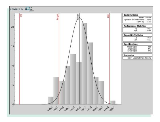
When a control chart of the process was produced, it became obvious that the manufacturer had not assessed process stability prior to calculating Cpk. In the control chart shown on the next page, you can see the process is not in control. Stability must be assessed before a capability study is done. Without this prerequisite, the Cpk statistics are not reliable.
