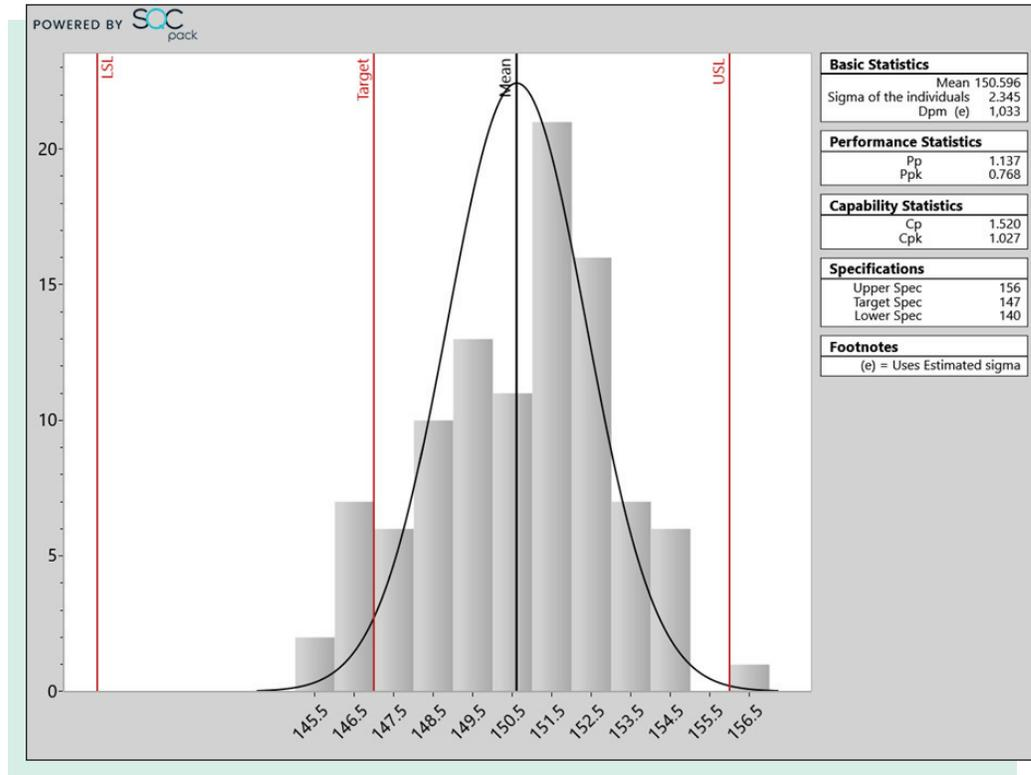
When a control chart of the process was produced, it became obvious that the manufacturer had not assessed process stability prior to calculating Cpk. In the control chart shown on the next page, you can see the process is not in control. Stability must be assessed before a capability study is done. Without this prerequisite, the Cpk statistics are not reliable.
