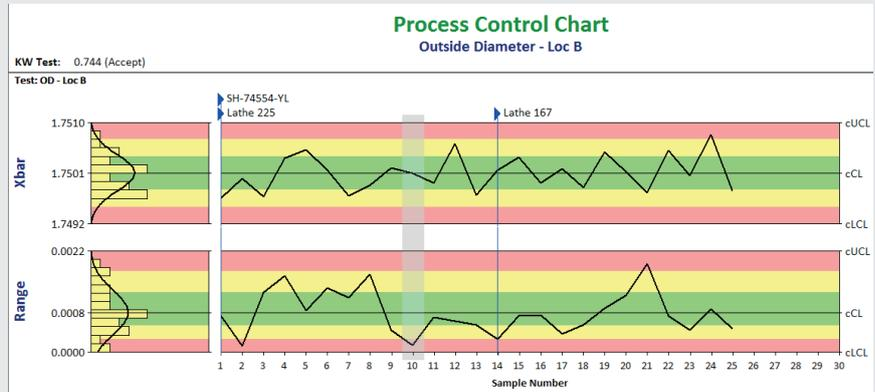
Figure 5. Charting a part run across two processes
