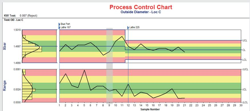
Figure 6. Automatic switch to accurate display of part run across two processes
